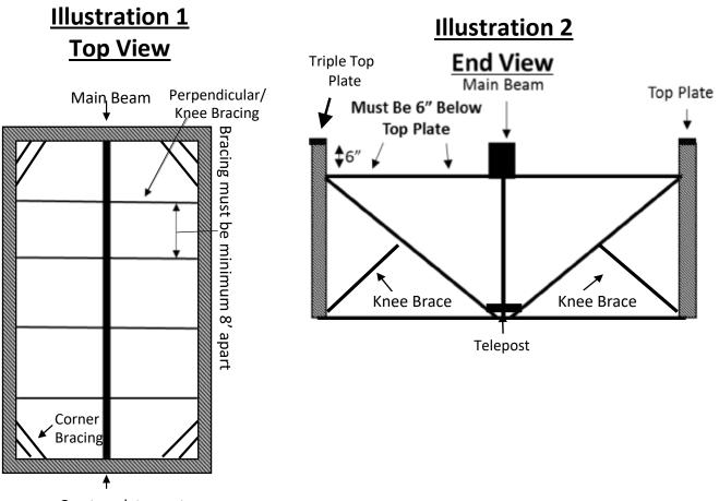
One top plate must run continuously through **CENTER** beam
