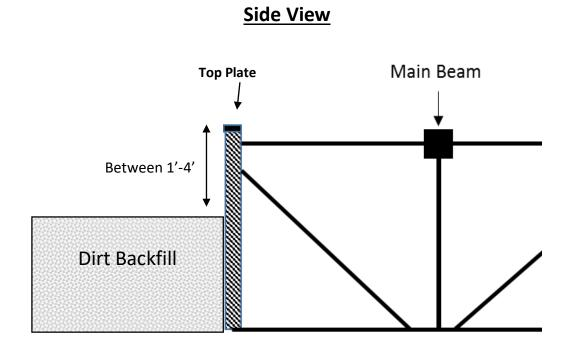
• All basements MUST be backfilled around the **ENTIRE** perimeter of foundation.
